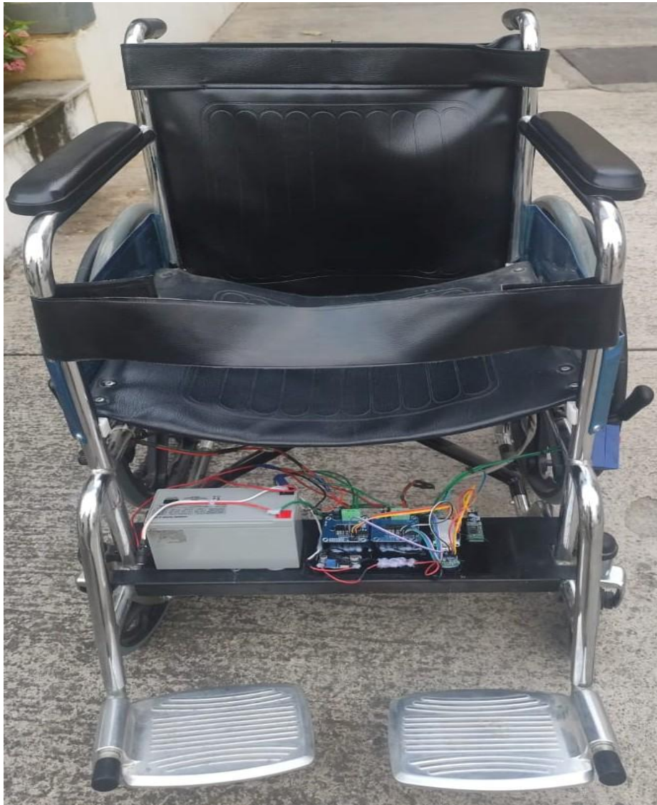
Fig 6.1: Result Of A Head, Bluetooth And Voice Controlled Wheelchair
