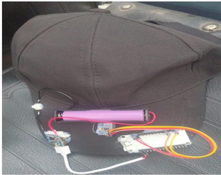
Fig 6.2: Result Of A Head Motion Control With Cap
